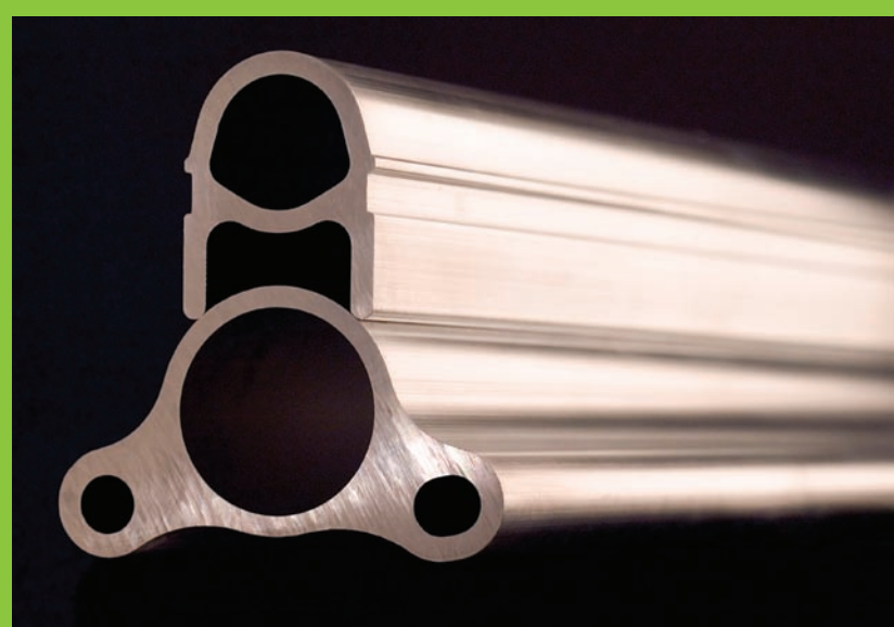
Kaiser Aluminum’s Sherman plant makes custom parts for end-use applications in the transportation market, including trailer components and truck parts.
