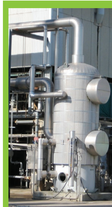
A loop dehydrator installed in ammonia plant #2 is also saving the plant 228,000 MMBtu per year.
